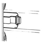
With door fully closed check that bolt slides through guide. Adjust hole if necessary.
