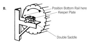
For Doors up to 3000mm High with Double Saddles through Bolts and Keeper Plates
