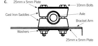
For doors over 3000mm high, rest axle between two cast iron
