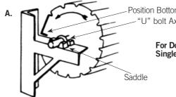
Position Bottom Rail here "U" bolt Axle Clamp
