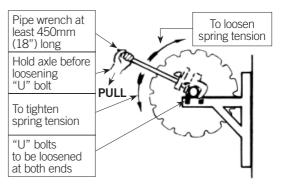
**WARNING:** Hold Axle before loosening "U" bolts. **IMPORTANT:** Do not attempt to loosen "U" bolts before securing firm hold on Axle with Pipe Wrench (stillsons). Do not use filters or similar brittle steel tools such as Tommy Bars.
