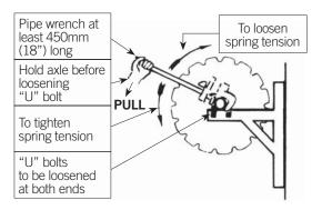
**WARNING:** Hold Axle before loosening "U" bolts. **IMPORTANT:** Do not attempt to loosen "U" bolts before securing firm hold on Axle with Pipe Wrench (stillsons). Do not use filters or similar brittle steel tools such as Tommy Bars.
