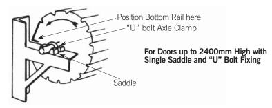
Rest axle on cast iron saddle. Immediately loosely secure with "U" bolts, nuts and washers, through slots in bracket arm. This eliminates the door falling from the brackets (See sketch).
