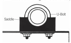
Before tightening "U" bolts, position the door so that it overlaps the opening evenly both sides so that the axle is positioned on the bracket arm slots as far forward as possible, while still allowing the bottom rail to pass the lintel when the door roll is rotated. Rotate both the door and the axle so that the bottom rail is level with the bracket arm. Now tighten the "U" bolts, using washers under nuts, to a torque of 40 newton metres or 30 ft.lb.
