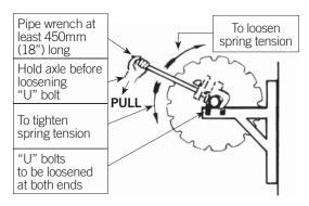
**WARNING:** Hold Axle before loosening "U" bolts. **IMPORTANT:** Do not attempt to loosen "U" bolts before securing firm hold on Axle with Pipe Wrench (stilsons). Do not use filters or similar brittle steel tools such as Tommy Bars.
