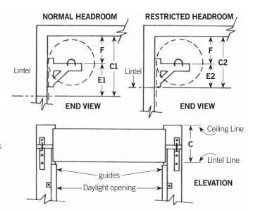
**NOTE:** Hand operated doors up to 2400mm high, the bottom rail will hang 65mm below lintel. For doors over 2400mm high bottom rail will be level with lintel.
