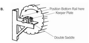
For Doors up to 3000mm High with Double Saddles through Bolts and Keeper Plates
