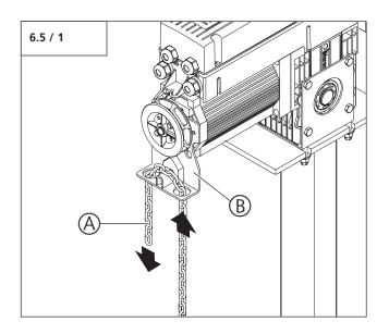
• Pull the emergency hand chain (A) through the entry on the motor unit (B).
