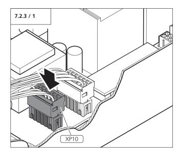
• Insert the plug of the cable loom into terminal XP10 (blue plug).
