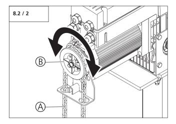
• Place the emergency hand chain (A) on the guide wheel (B).
