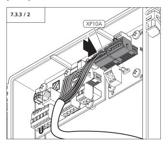
• Insert the plug of the cable loom into socket XP10A (blue plug).
