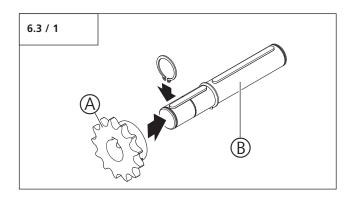
• Fit the sprocket (A) to the drive shaft assembly (B).
