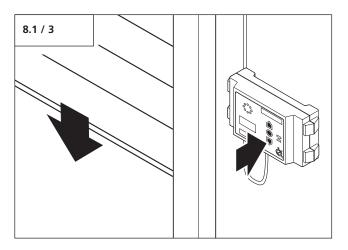
• Press the CLOSE button on the Control x.plus control unit.
