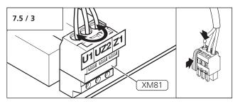
• At the motor connection (XM81), swap lead (U1) with lead (Z1).
