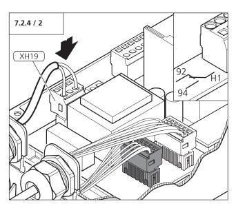
• Insert the plug of the devices to be connected into socket XH19.
