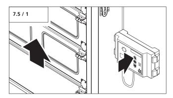
• Press the OPEN button on the control unit.
