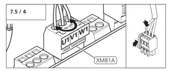
• At the motor connection (XM81A), swap lead (U1) with lead (W1).
