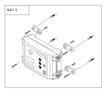
• Mount the Control x.plus control unit on the same side as the motor unit.
