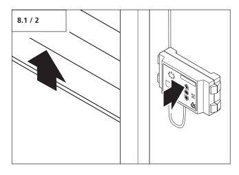
• Press the OPEN button on the Control x.plus control unit.
