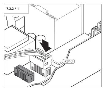
• Insert the plug of the cable loom into terminal XB40 (white plug).
