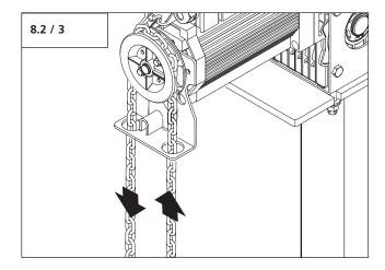
• Move the door in the OPEN or CLOSE direction by pulling on the emergency hand chain.
