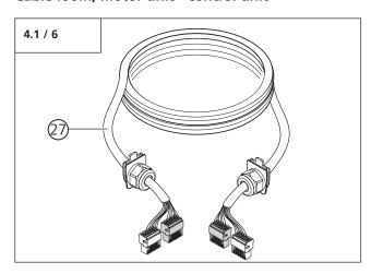
27 Cable loom, motor unit - control unit
