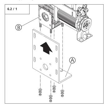
• Screw the motor unit console (A) to the motor unit (B).
