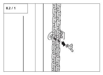
• Release the emergency hand chain from the securing assembly.
