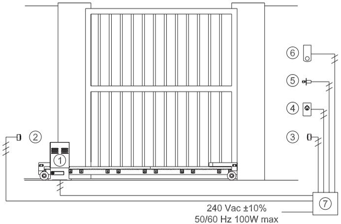
**NOTE** The Merlin M122 wired pushbutton and M128 wireless pushbutton are not waterproof, and are only rated for interior use.
