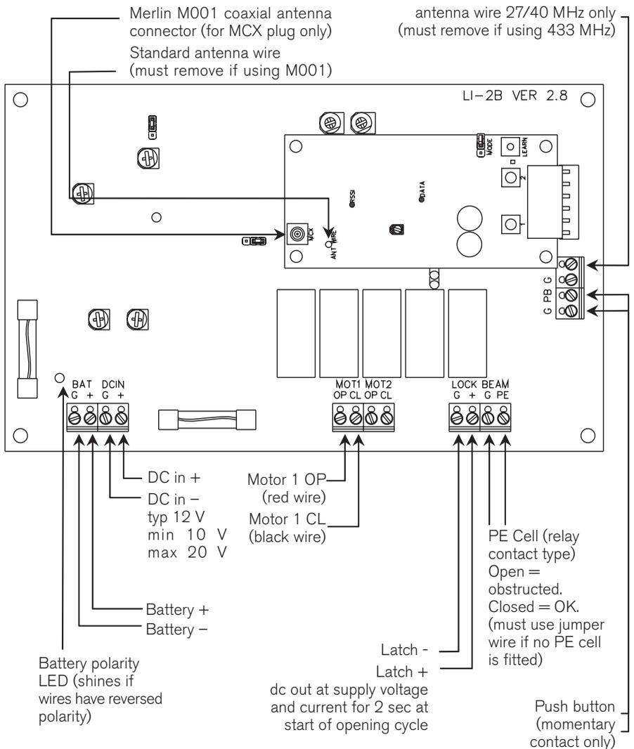
**NOTE** When powering any accessories from the board, (for example: gate latches, additional receivers, keypads, PE beams) ensure the power supply has adequate capacity. Measure the voltage at DC IN under full motor load. If it falls below 9 V dc then the board, receiver, and some accessories, may not function correctly. In this instance, remove accessories, upgrade the power supply, or provide additional power supplies directly to each accessory.
