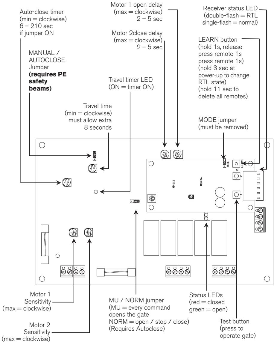
**NOTE Reverse motor wires if open and close LEDs don't match gate travel.**
