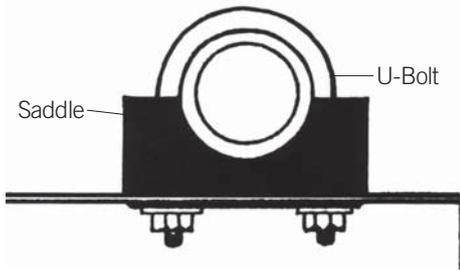
Before tightening "U" bolts, position the door so that it overlaps the opening evenly both sides so that the axle is positioned on the bracket arm slots as far forward as possible, while still allowing the bottom rail to pass the lintel when the door roll is rotated. Rotate both the door and the axle so that the bottom rail is level with the bracket arm. Now tighten the "U" bolts, using washers under nuts, to a torque of 40 newton metres or 30 ft.lb.
