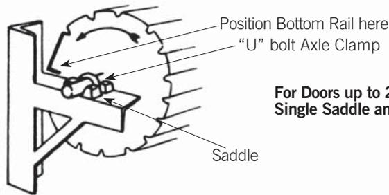
**For Doors up to 2400mm High with Single Saddle and "U" Bolt Fixing**
