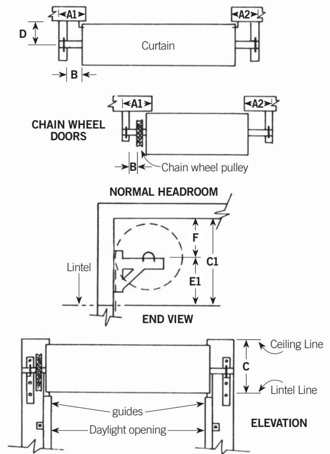
**NOTE:** Hand operated doors up to 2400mm high, the bottom rail will hang 65mm below lintel.
